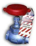
**Tagout:** The practice of using tags in conjunction with locks to increase the visibility and awareness that equipment is not to be energized or activated until such devices are removed. Tags are non-reusable, attachable by hand, self-locking, and not easily removed.
